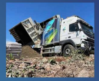
The right-hand tipping unit is an industry standard specification. This permits for the hydraulic power arm to be positioned on the left-hand side of the vehicle, allowing for superior reach when excavating.
