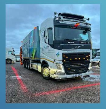
Collaborating with FHOSS, the global innovators in illuminated safety solutions, SEUK has co-designed the ultimate segregation solution for Suction Excavators which not only provides a clear 360 degree visual exclusion zone, but also uses AI cameras to detect, audibly warn, and record pedestrian excursions into the danger zone. This enables us to both prevent accidents and change pedestrian/operator behaviour.
