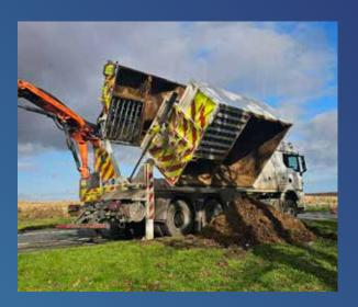
The right-hand tipping unit is an industry standard specification. This permits for the hydraulic power arm to be positioned on the left-hand side of the vehicle, allowing for superior reach when excavating.
